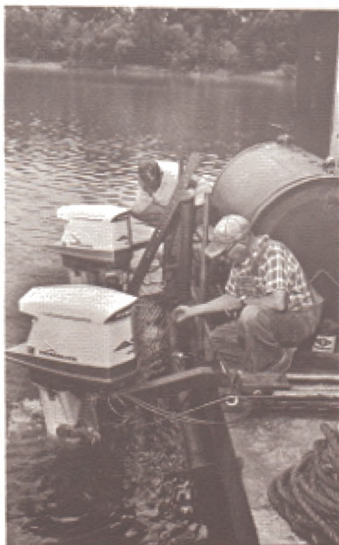
A specially designed rigging was devised for these two Homelite engines to fit them for the tough job of powering a 40,000 pound barge, used to dredge out mussels
