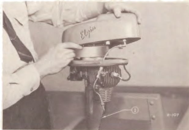
FIGURE 2 - REMOVING FUEL TANK 1. Idle Relief Holes
