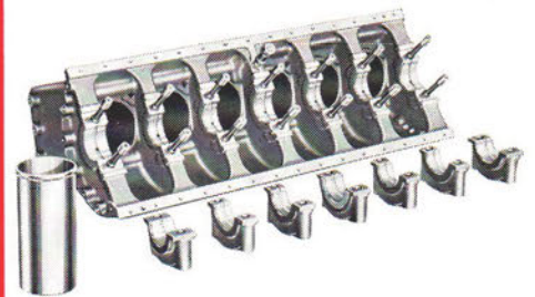
Cylinder block (showing main bearings, caps and cylinder sleeve).
